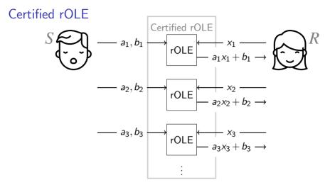
Sender can prove  $(a_1, b_1, a_2, b_2, ...)$  satisfies arithmetic constraints  $a_i = a_j$  for some (i, j) for general constraints  $\rightarrow$  see eprint
